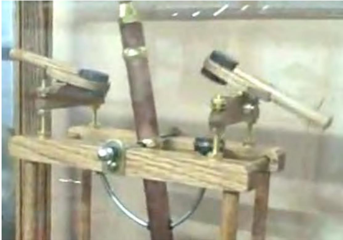
Presumably, the arm is curved to avoid the constructional complications at the pendulum pivot which would be caused by a straight mounting arm attached to the pendulum shaft. The rising magnet attached to the pendulum pushes the magnet end of the rocker arm upwards even though it does not come close to it.
