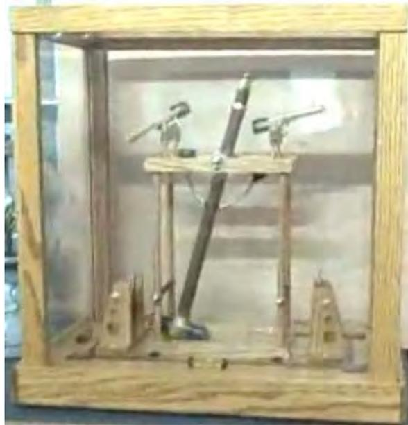
Which indicates the swing covers a fairly short distance. Mounted near the top of the pendulum, there are two pivoted arms which look quite like microphones, due to having large magnets mounted on their innermost ends:
